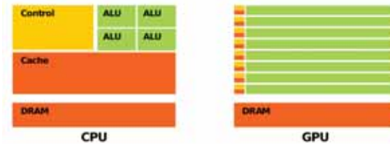
Figure 2: Basic structure of a typical CPU (left) and GPU (right).
