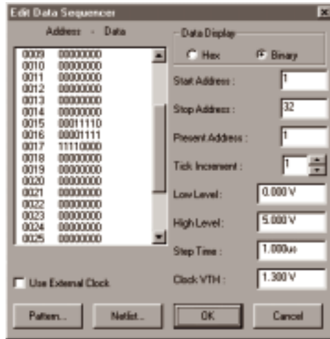
Figure 5.6. Use the Edit Data Sequencer dialog box to edit stimulus for your circuits.
