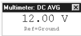
Figure 6.12. The Multimeter showing the DC operating point of a point in the circuit.
