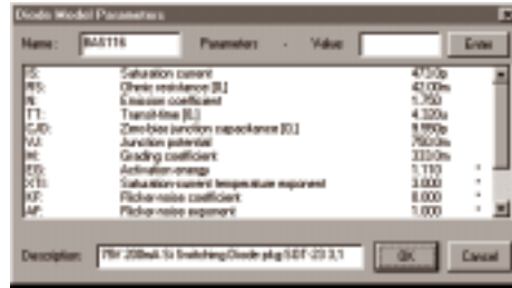
Figure 16.12. Use the Diode Model Parameters dialog box to change the settings of a particular model.
