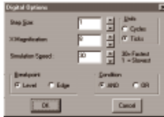
Figure 5.1. Use the Digital Options dialog box to specify the size of a step and other digital simulation options.
