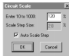
Figure 13.2. This dialog box controls the scale of the displayed circuit and the scale step of the Zoom Tool.
