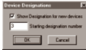
Figure 12.1. Use this dialog box to specify designation options for new devices you place in the schematic.
