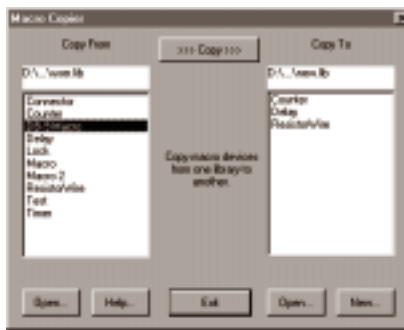
Figure 11.4. Use this dialog box to copy macros from one macro library to another.
