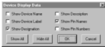
Figure 12.2. Use the Device Display Data dialog box to quickly change the display settings of all selected devices.
