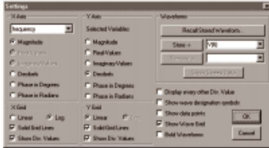
Figure 6.5. Use the Settings dialog box to control the X and Y axes of the graph, to store and recall waveforms and to alter the visual aspects of the analysis window.
