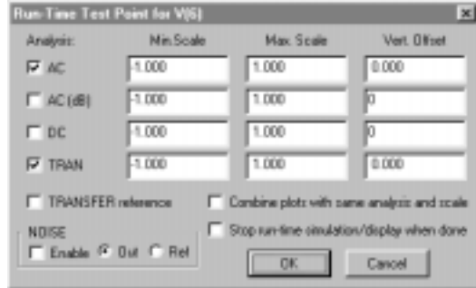
Figure 6.28. Use this dialog box to set up Run-Time Test Points for the nodes you want to observe (right-click with the Probe Tool on a point in the circuit).
