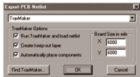
Figure 7.3. Not only can you export a TraxMaker netlist, but you can also launch TraxMaker, load the netlist, and automatically define a keep out area and place the components, all from within CircuitMaker.
