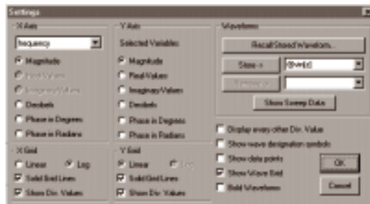
Figure 6.31. For Impedance Plots, you would normally change the Y axis to Magnitude. Click the Settings button in the analysis window to change X and Y axes for that window.
