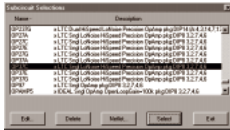
Figure 3.10. Use the Subcircuit Selections dialog box to select a specific model, such as the UA741.
